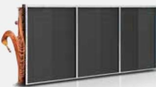
Hydrophilic finned block heat exchangers are installed; these break down the drops of water into particles and reduce the obstruction of the space between one fin and another caused by ice build-up. Thanks to a lower surface tension, the water tends to slide and precipitate by gravity, preventing the formation of frost at low temperatures.
